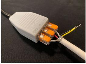
Figure 10 Connecting data to USB up-loader cable for POI fixtures
