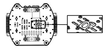
Figure 5: Safety Wire attachment point
