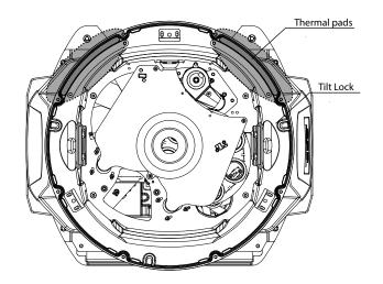
Figure 32 Thermal pads to be replaced
