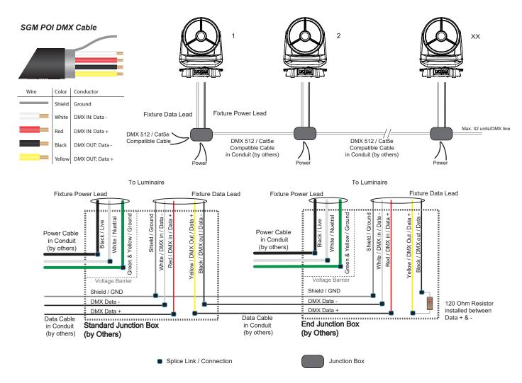
Figure 16: Connecting DMX and AC Power in G-7 BeaSt POI
