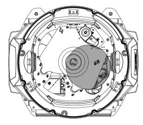
Figure 26: The gobo is under the marked area
