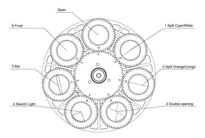
Figure 22: Identification of gobo wheel
