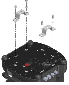
Figure 15: Omega bracket attachment
