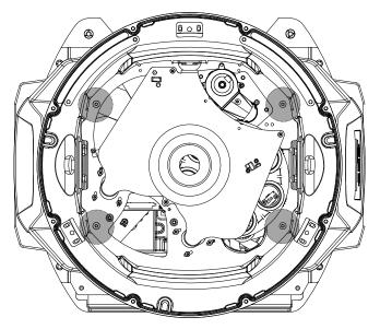
Figure 36: Illustration of screws for BeaSt module
