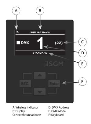
Figure 17: Control panel view
