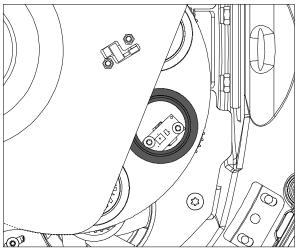
Figure 27: Turn the gobo to the position which is to be replaced  $% \left( 1\right) =\left( 1\right) \left( 1\right) \left($
